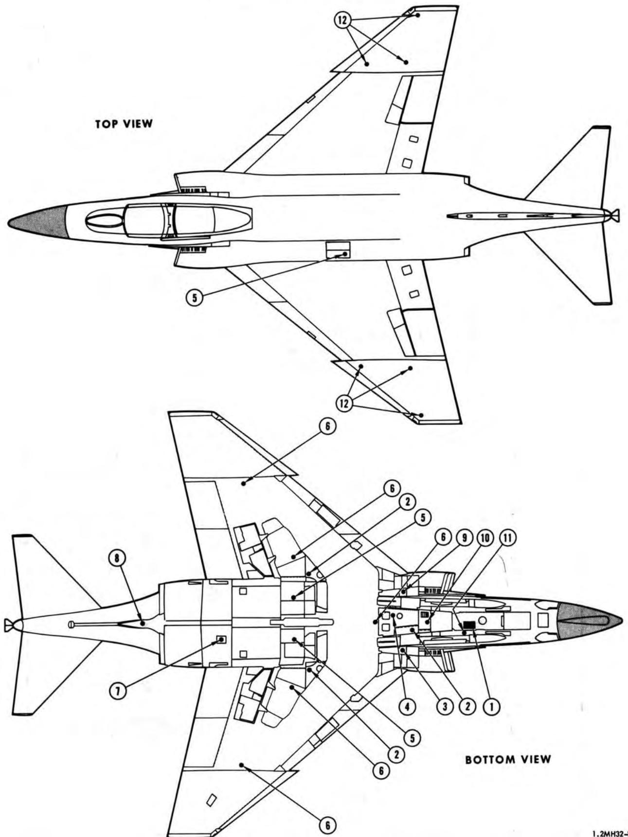
Figure 6-11. Servicing and Precaution Markings (Sheet 1)
